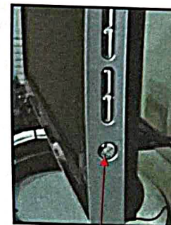
Power SW of Monitor
