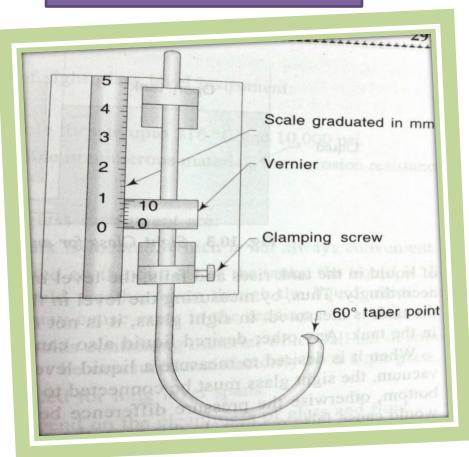
• The level of liquid in an open tank is measured directly on a scale
