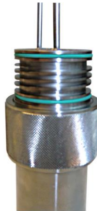
Fig. 28. Water cooling O-rings.
