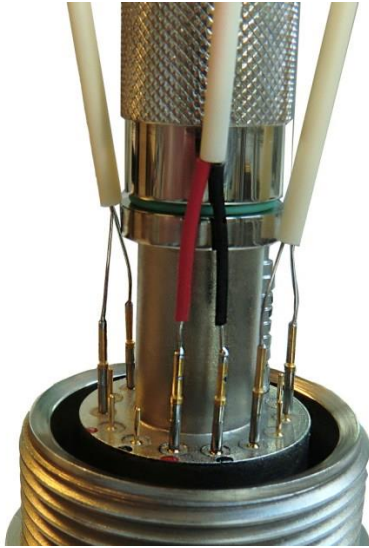
Fig. 21. The S-type thermocouple mounted in the S-wired base unit.
