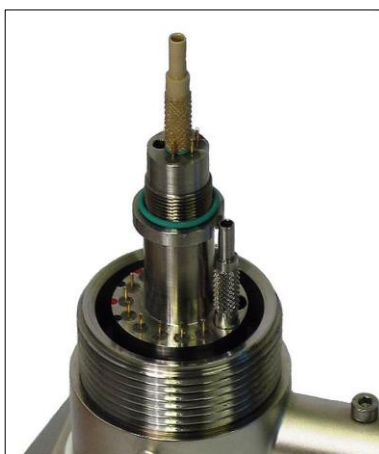
Figure 4-3: Base unit with pedestal. Version A-6 with replaceable gas stubs. On the pedestal: Gas inlet and outlet and 4 feedthroughs. Further down: Inner O-ring. On the base circle: Gas inlet and outlet and 12 feedthroughs.
