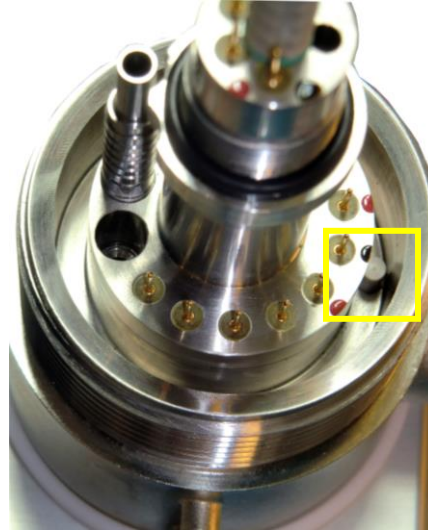
Picture 5. The stopper inserted in the hole.
