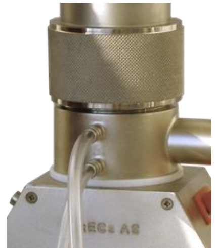
Fig.29. Cooling water connected.
