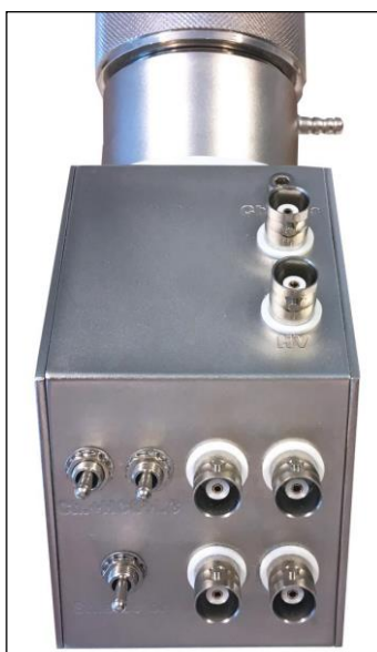
Figure 4-8: 6 individual BNC connectors. Shields bridge, Ch+HCS and LC+HCS switches (connects when down).
