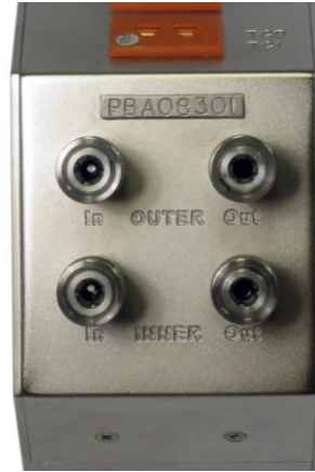
Fig. 2: IN and OUT quick-connects for INNER and OUTER gas compartments.
