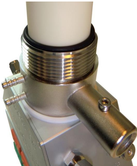
Picture 6. Outer alumina tube inserted.
