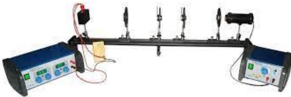
Fig.-(1) Experimental setup for recording the current-voltage characteristics of a CdS photoresistor.
