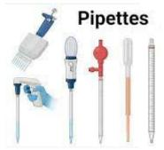
**PIPETTE :** Pipette is a glass tube used for the delivery of a measured quantity of liquids.
