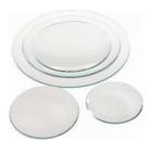
**WATCH GLASS :** Watch glass is used to allowcrystal to dry after they have been filtered. They canbe used as an evaporating surface or to cover a beaker that can be heated to very high temperatures.
