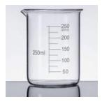
**BEAKER** : A beaker is a cylindrical glass or plastic vessel used for holding liquids. It is a multi- purpose piece of equipment used for containing a chemical reaction, measuring liquids, heating them over a Bunsen burners flame or collecting them in a titration experiment.
