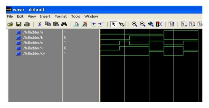
**Results:**VHDL codes of full adder is simulated & synthesized
