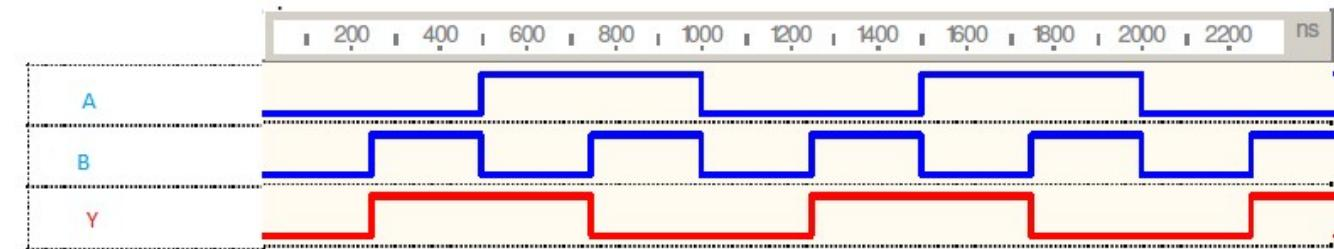
g) XNOR Gate: A logic gate that produces logic ‘1’ only when the two inputs are equal.
