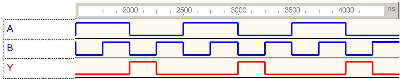
f) **XOR Gate:** A logic gate whose output is logic ‘0’ when all the inputs are equal and logic ‘1’ when they are unequal.
