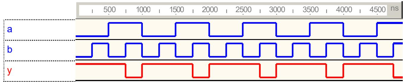
e) NOR Gate: A logic gate whose output logic is ‘1’ if and only if all of its inputs are logic ‘0’
