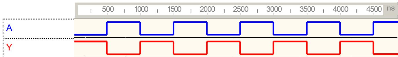
d) **NAND Gate:** A logic gate which gives logic ‘0’ output if and only if all of its inputs are logic ‘1’
