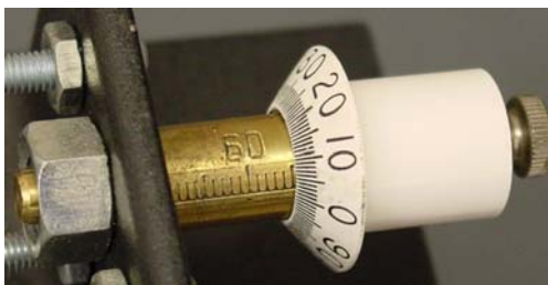
Figure 2 Close-up of the micrometer screw at one end of the apparatus. The brass barrel is marked in cm (stamped numbers) with tick marks every mm. the dial allows measurement of 0.01 mm with index being the horizontal line marked on the brass barrel.
