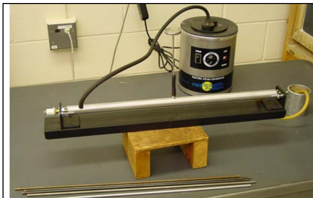
Figure 1 The linear expansion apparatus. The rods are placed inside the silver jacket and the whole assembly is placed on the black base.
