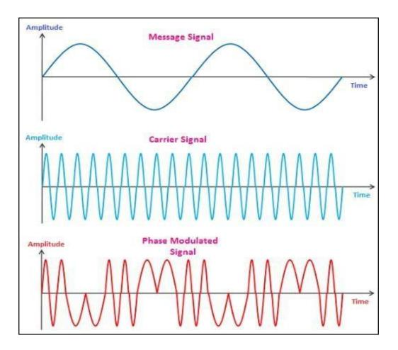
Fig. The output of Phase Modulation.
